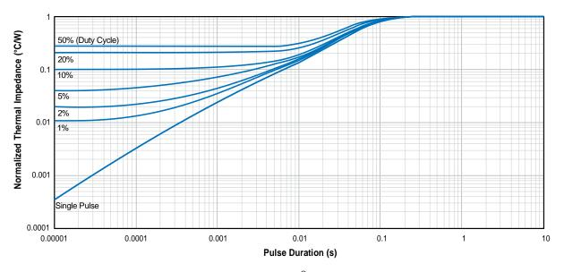
Figure 30. Typical Low- or High-Side Power eGAN® HEMT Normalized Junction-to-Case Thermal Impedance
