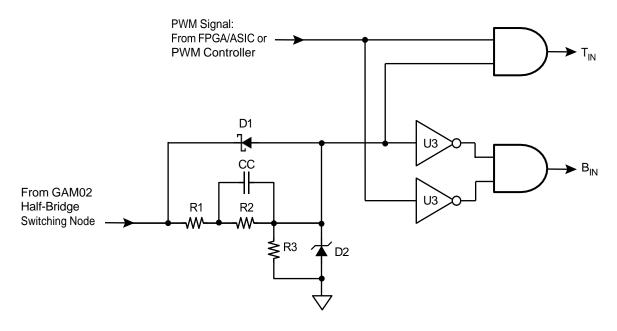
Figure 17. Adaptive Dead Time Control for Cross-Conduction/Shoot-Through Avoidance
