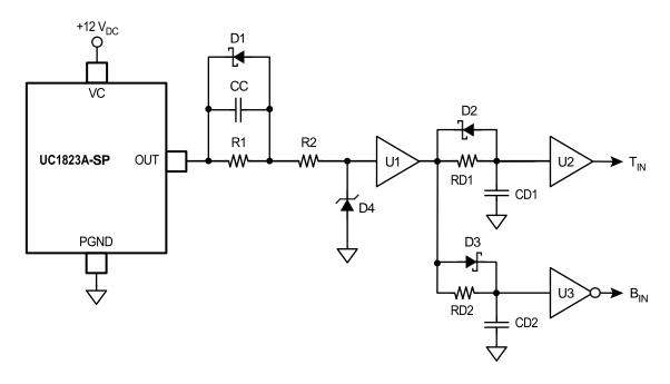
Figure 15. Zener Diode Logic Input Voltage Clamp Circuit and Dead Time Delay Circuit
