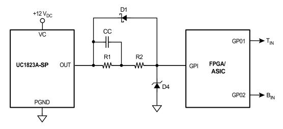
Figure 16. Zener Diode Logic Input Voltage Clamp Circuit with ASIC/FPGA Two-Phase Clock (With Dead Time) Generator
