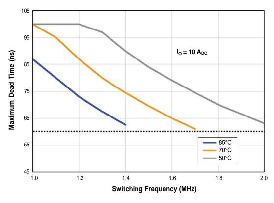
Figure 29. Maximum Dead Time  $(t_{dt})$  vs. Switching Frequency  $(f_{sw})$  vs. Module Case Temperature  $(T_c)$ ,  $I_o = 10$  A, Half-Bridge Configuration (Refer to Fig. 21).
