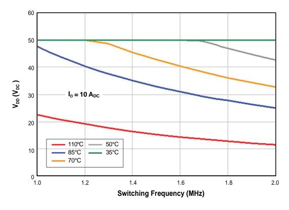
Figure 25. Maximum Switching Frequency vs. Supply Voltage ( $V_{DD}$ ) vs. Module Case Temperature ( $T_c$ ),  $I_o = 10$  A, Half-Bridge Configuration.
