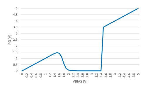
Figure 6. Typical PG Output vs  $V_{BIAS}$  Input
