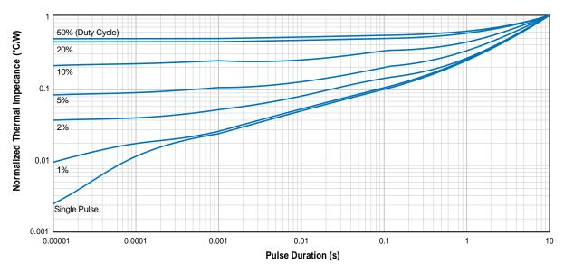
Figure 31. Typical Low- or High-Side Catch Schottky Normalized Junction-to-Case Thermal Impedance
