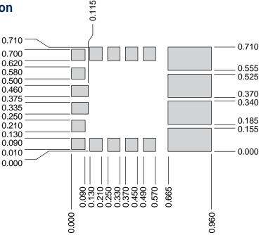
Figure 33. Recommended PCB Solder Pad Configuration (Top View)
