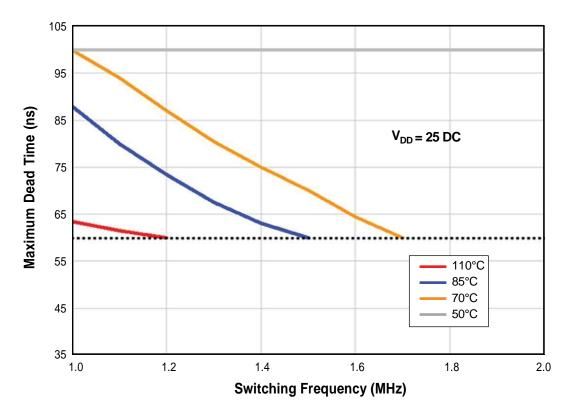
Figure 28. Maximum Dead Time  $(t_{dt})$  vs. Switching Frequency  $(f_{sw})$  vs. Module Case Temperature  $(T_c)$ ,  $V_{DD} = 25 \ V_{DC}$ , Half-Bridge Configuration (Refer to Fig. 23).
