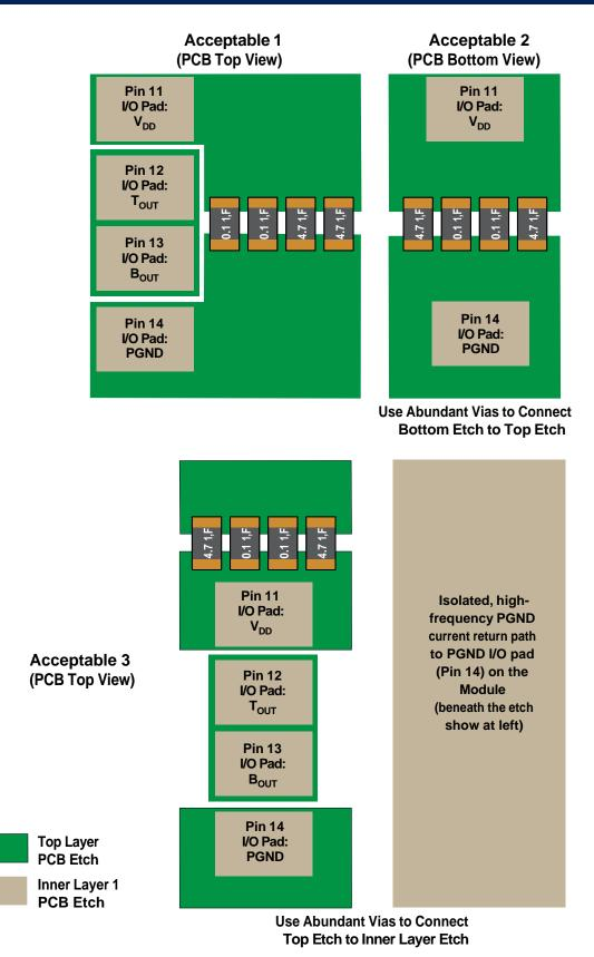
Figure 22. Recommended V<sub>DD</sub>-to-PGND Power Supply Bypassing (Not to Scale)
