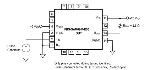
Figure 1. T<sub>IN</sub>-to-T<sub>GATE</sub> Switching Time Test Circuit
