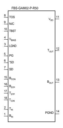
Figure 23. Suggested FBS-GAM02-P-R50 Schematic Symbol
