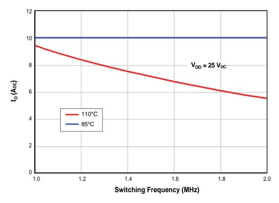
Figure 27. Maximum Output Current ( $I_o$ ) vs. Switching Frequency ( $f_{sw}$ ) vs. Module Case Temperature ( $T_c$ ),  $V_{DD} = 25 \ V_{DC}$ , Half-Bridge Configuration.
