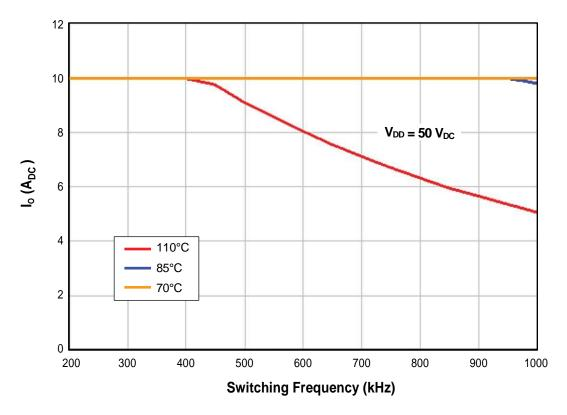
Figure 26. Maximum Output Current ( $I_o$ ) vs. Switching Frequency ( $f_{sw}$ ) vs. Module Case Temperature ( $T_c$ ),  $V_{DD}$ = 50  $V_{DC}$ , Half-Bridge Configuration.
