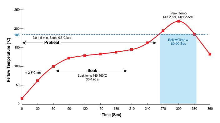
Figure 34. Sn63/Pb37 No Clean Solder Paste Typical Reflow Example Profile.
