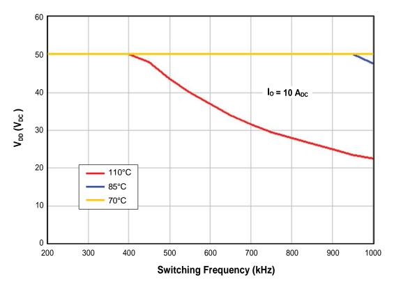
Figure 24. Maximum Switching Frequency vs. Supply Voltage ( $V_{DD}$ ) vs. Module Case Temperature ( $T_c$ ),  $I_o = 10$  A, Half-Bridge Configuration.
