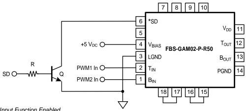
Figure 20. \*SD Input Function Enabled
