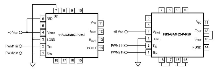
Figure 18. PG Protection Functions Disabled
