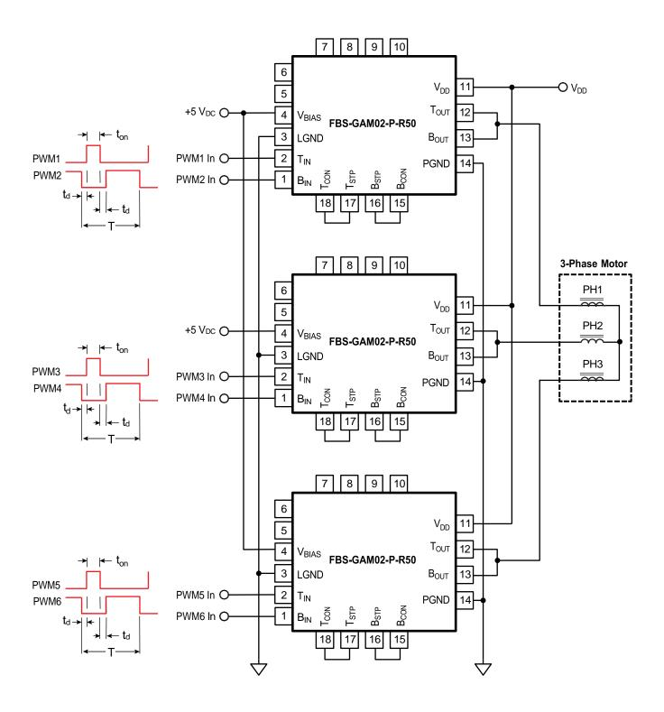
Figure 14. Half-Bridge Configuration: Three Phase Motor Drive Stage
