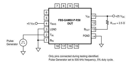
Figure 3. B<sub>IN</sub>-to-B<sub>OUT</sub> Switching Time Test Circuit
