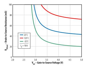
Figure 8.  $R_{DS(on)}$  vs.  $V_{GS}$  for Various Temperatures
