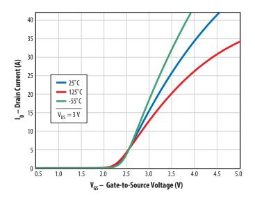
Figure 5. Typical Transfer Characteristics
