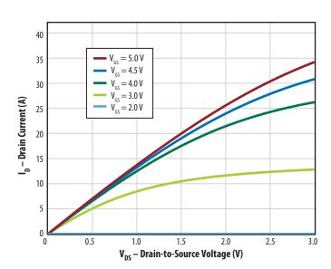
Figure 4. Typical Output Characteristics at 125°C
