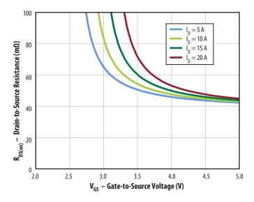
Figure 7.  $R_{DS(on)}$  vs.  $V_{GS}$  for Various Drain Currents
