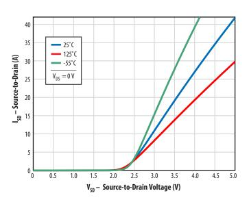
Figure 6: Reverse Drain-Source Characteristics
