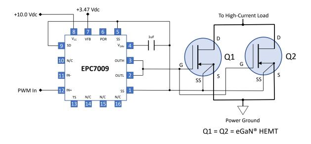
Note: Make all OUTH/OUTL-to-Gate, SS-to-Source Sense and Source connections as short as possible. Also keep the Drain connections as short as physically possible.
