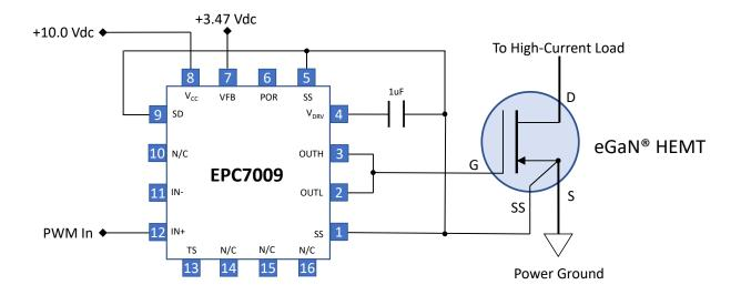
Note: Keep Out-to-Gate and SS-to-Source-Sense connections as short as possible.
