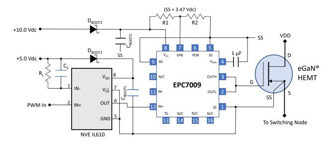
Note: Make all OUTH/OUTL-to-Gate, SS-to-Source Sense and Source connections as short as possible. Also keep the Drain connections as short as physically possible. The SS node may be treated as a local etch plane in the area of the IL610, the EPC7009 and the eGaN® HEMT. Circuit shown utilizes dual bootstrapping: one for the NVE IL610 and one for the EPC7009.
