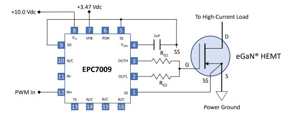
Note: Make all OUTH-to-RG1, OUTL-to-RG2, the tie point of RG1/RG2-to-Gate and SS-to-Source Sense connections of equal length and as short as possible. RG1/RG2 are 20  $\Omega$ , maximum
