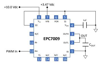
Only pins connected during testing identified. Pulse Generator set to 500 kHz frequency, 5% duty cycle.
