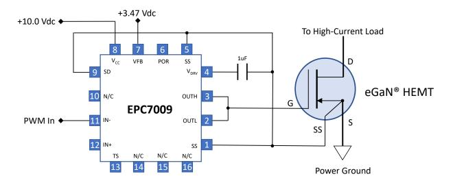
Note: Keep Out-to-Gate and SS-to-Source-Sense connections as short as possible. *Figure 8. Inverting Mode Low-Side Driver and EPC Space eGaN® HEMT*
