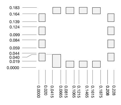
Figure 13. Recommended PCB Solder Pad Configuration (Top View)
