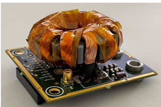
Figure 14: EPCS401 with air-core 220nH inductor.
